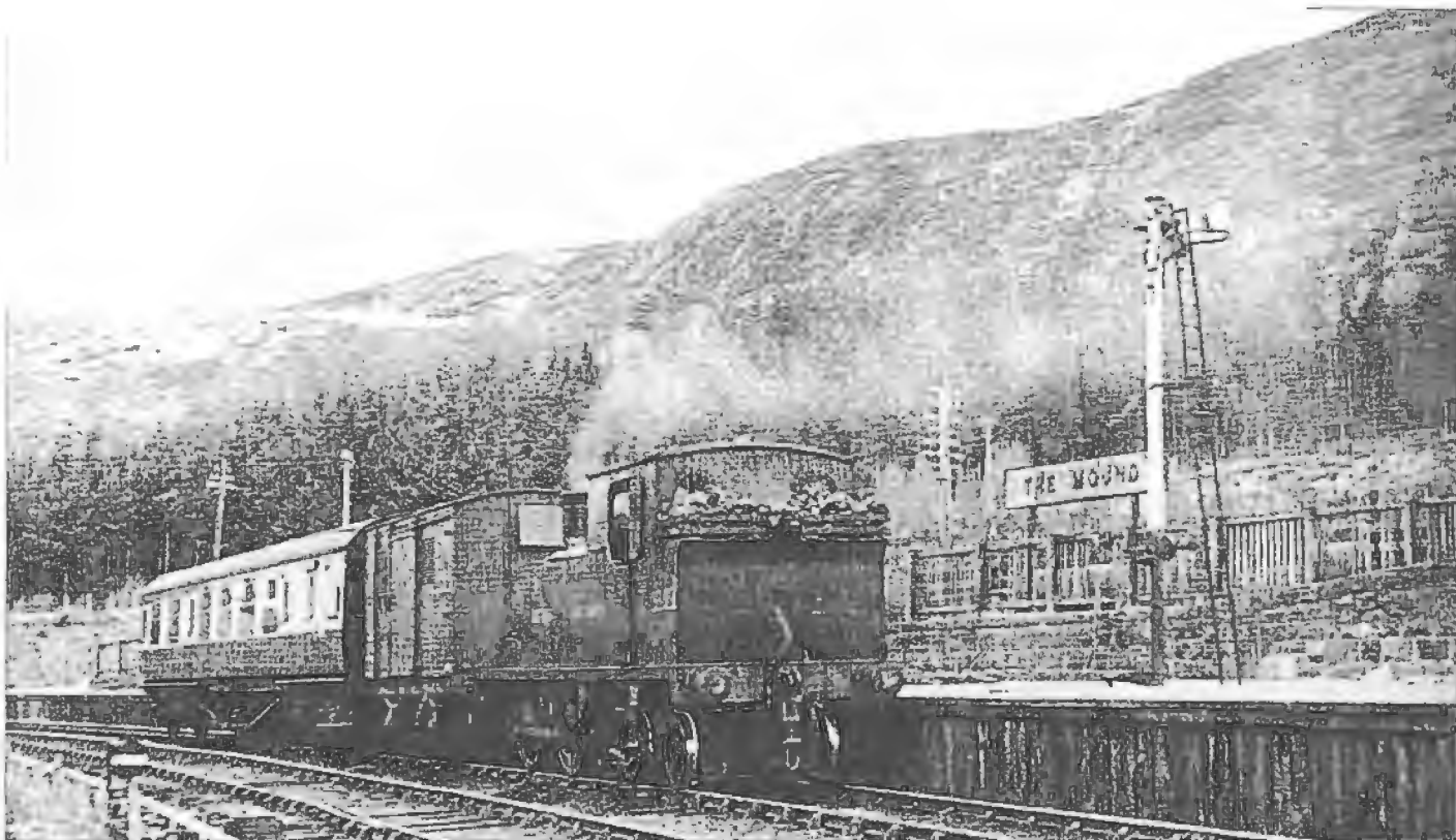
Clearly, the station at The Mound did not serve a bustling centre of population. On 23 April 1952 No.55051 waits to depart from the somewhat isolated station with the 11.55am to Dornoch. The coach is brake corridor compo SC6755M, one of a batch of twenty-five 60ft coaches built at Wolverton in 1930. It was not originally flush-sided - rebuilding took place circa 1940 when it received 'Period III' panels and deep window ventilators. PHOTOGRAPH: H.C.CASSERLEY
