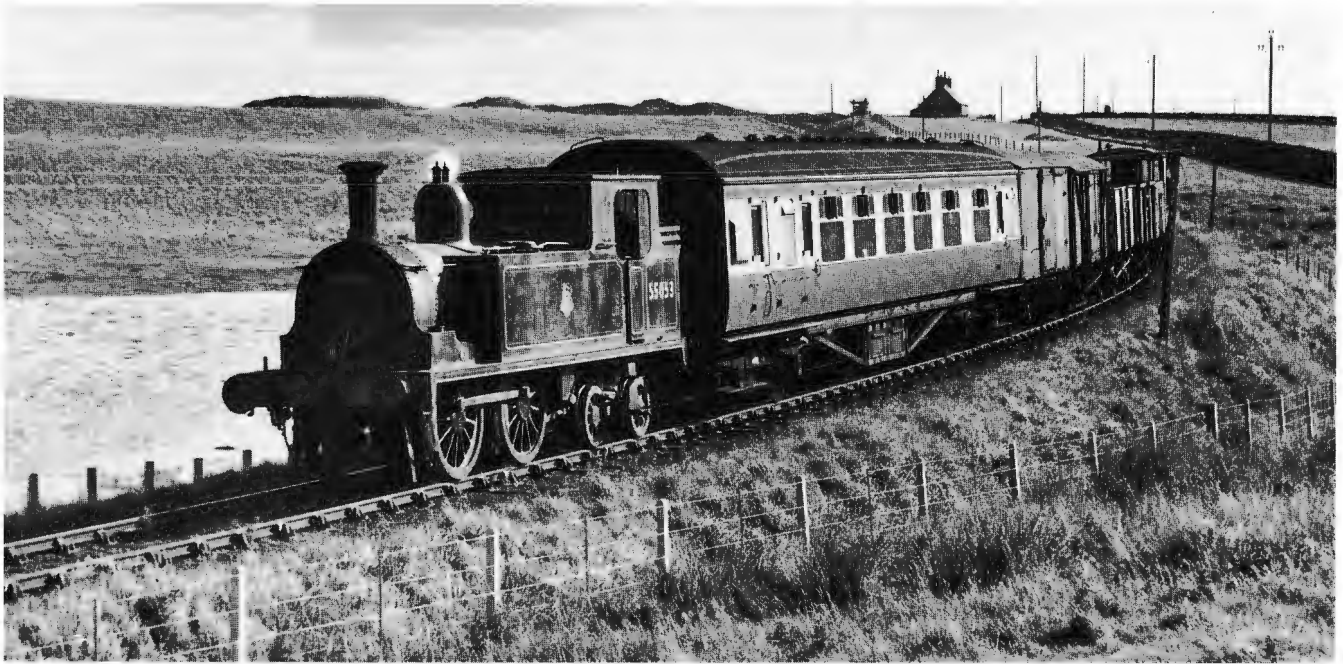
Above: In 1956, the 1.00pm Dornoch to The Mound mixed train makes sedate progress, not long after departure from the terminus. The engine is Drummond 0-4-4T No 55053, in its last year of service. Behind the engine is one of the re-panelled LMS corridor brake composites of the 1920s that were modernised in the 1930s and seemed to be favourites for service in northern Scotland. W. J. Verden Anderson/Rail Archive Stephenson
