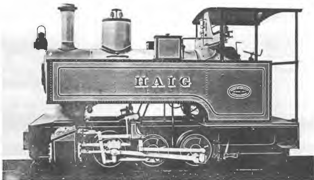
Kerr Stuart photographed the prototype Haig 0-6-0T (KS 3083/17) specially painted and lettered with the class name before delivery. Although none were built for UK customers after the 1914/18 War, it proved a popular loco overseas, primarily for sugar cane tramways, and indeed four more were built by Bagnall after Kerr Stuart's demise in 1930. (Hunslet Engine Co./Armley Museum, Leeds)
